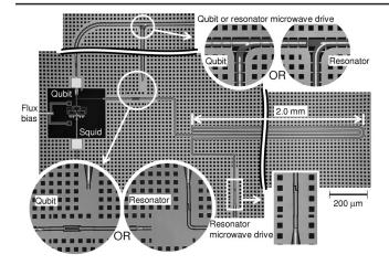
FIG. 1. Photomicrograph of a coplanar waveguide resonator coupled to a phase qubit. The total length of the half-wavelength resonator is 8.8 mm. The insets show the two designs of the microwave lines that were varied in fabrication to connect the resonator either to a qubit or a classical preamplifier, allowing qubit-based  $T_1$  or classical resonator Q measurements, respectively. Square holes in the ground plane are to immobilize trapped vortices.
